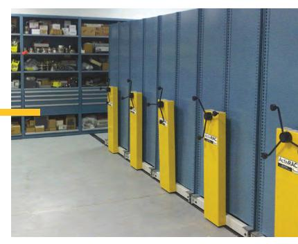
The ActivRAC<sup>®</sup> 8M system has ergonomically designed handles and a mechanical-assist drive unit on each carriage.
