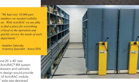
The ActivRAC 8M system consisted of five rows of mobile carriages with two static ends cabinets. A single 3.5' aisle maximized storage density.
